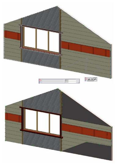
All other top and bottom shapes (excluding Follow Wall) can also be edited dynamically. The object interface also provides an 'offset' parameter to allow the top and bottom shape to be easily offset.
