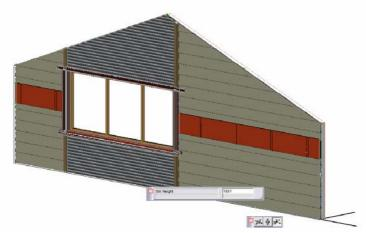
If the custom setting is used for the top and bottom shapes, dynamic hotspots are added to the midpoints of edges so the actual shape can be edited dynamically.
